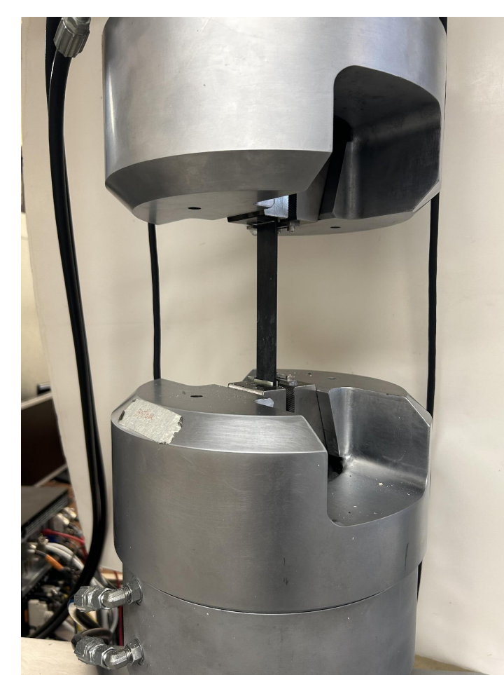
Tensile coupon testing on the Instron [Left]
