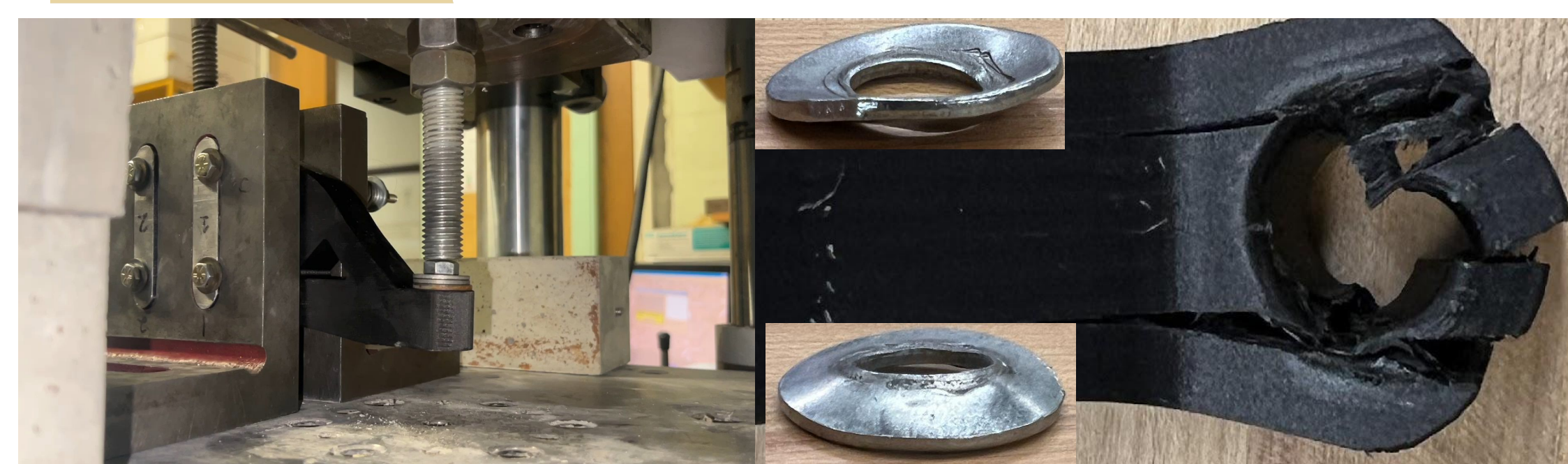
Testing Apparatus (Left) Iteration V (Test I)[Right]: Local failure caused by cupping of washer
