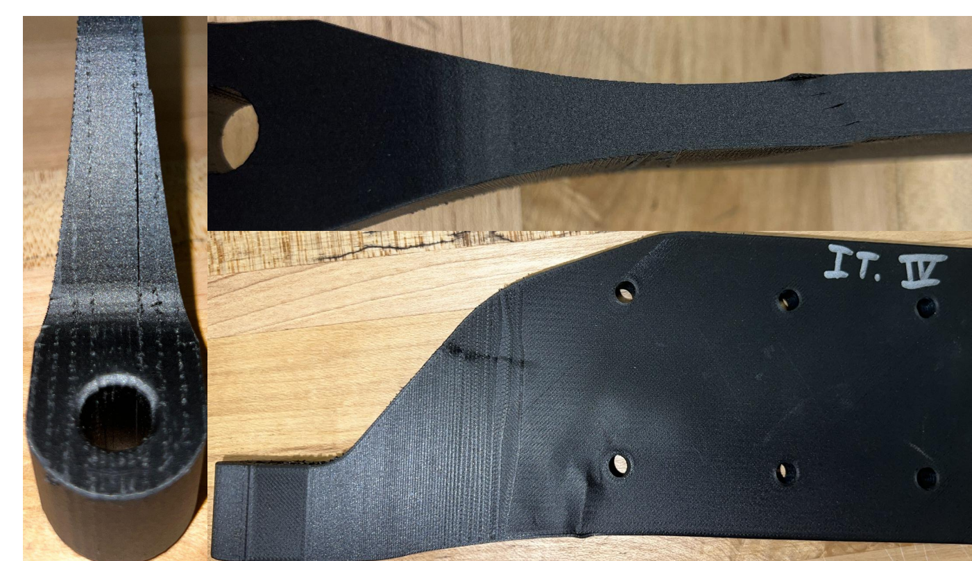
Iteration IV (Left): Combined shear, tensile, and buckling failure Iteration V (Test I) [Right]
